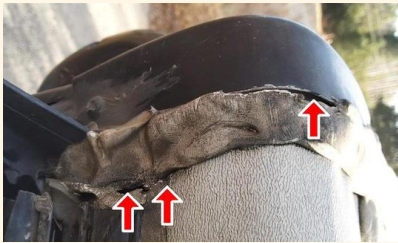
Curbside Rear Roof Sealant Gap
