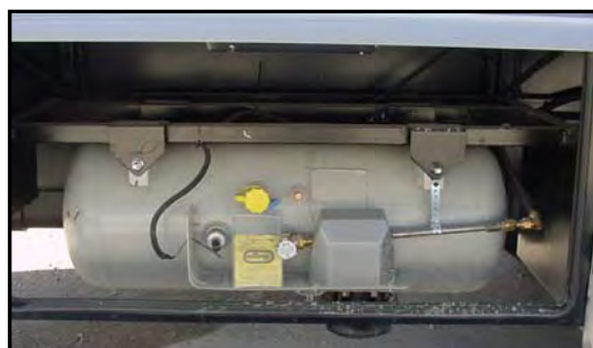
Figure 2-2. Liquid Propane Tank
