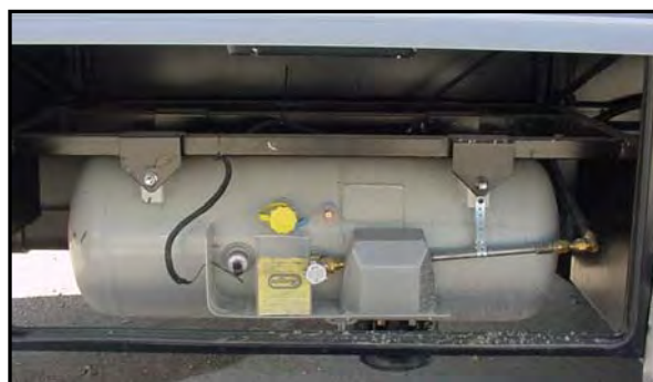
Figure 2-4. Liquid Propane Tank
