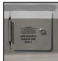
Figure 2-3. Fuel Tank Fill Door
