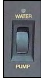
Figure 11-5. Water Pump Switch
