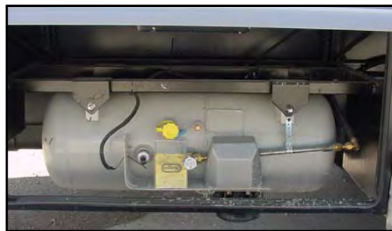
Figure 3-5. Liquid Propane Tank
