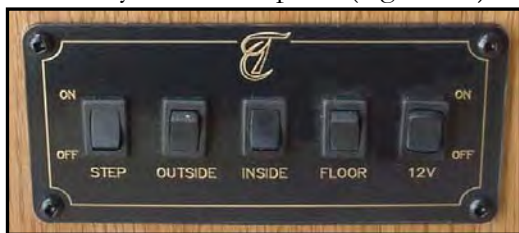
Figure 7-4. Battery Disconnect Panel
