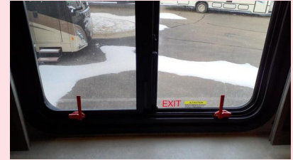
Bedroom Emergency Exit Window
