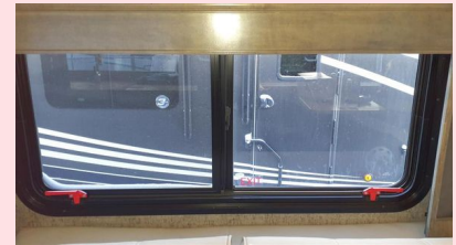
Emergency Exit Window
