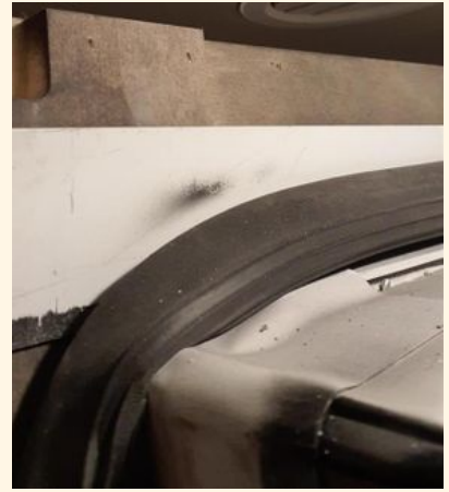
Curbside Rear Inside Seal will miss the wall
