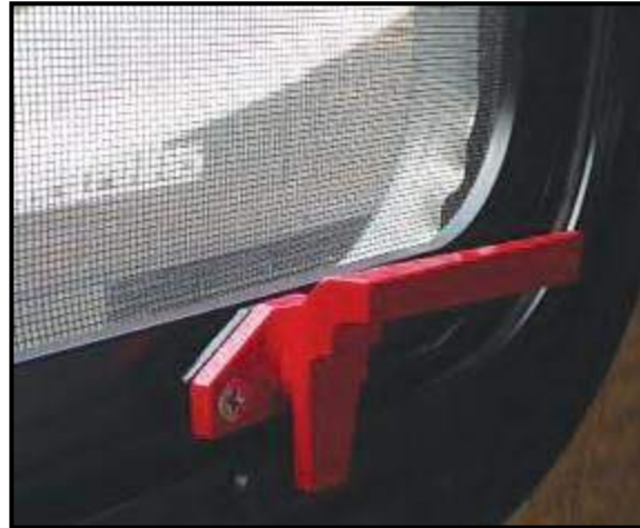
Figure 2-9: Emergency Exit Latch
