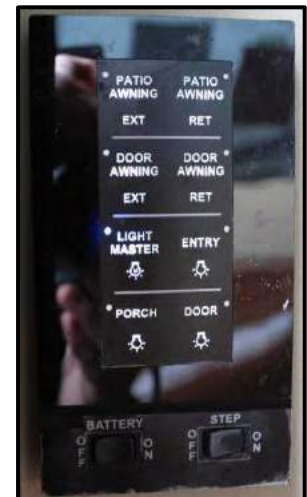
Figure 9-16: 12 VDC Disconnect Switch
